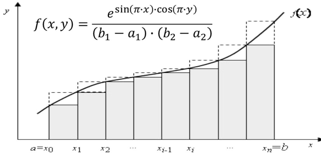
$$\int_a^b f(x) dx \approx \frac{b-a}{n} (y_0 + y_1 + \dots + y_{n-1}) = \frac{b-a}{n} \sum_{i=0}^{n-1} f(x_i)$$
