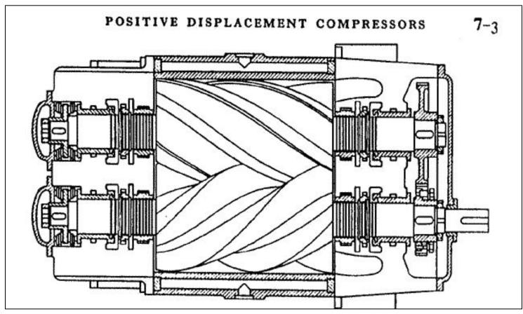
Contact of screws of rotors is not permissible, therefore, a minimal clearance is provided between them, which ensures the safe operation of the compressor.
