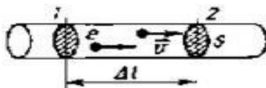
$$\Delta Q = eN, \Delta l = \bar{v}\Delta t, N = nV, V = S\Delta l,$$
