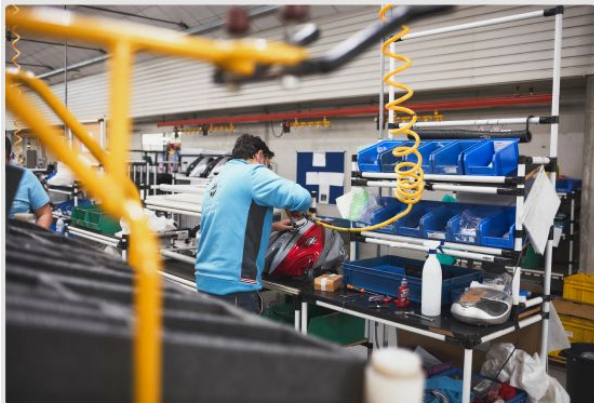
SIMILARLY, THE SO-CALLED "SUPERMARKET" AREA IS WHERE ALL THE NECESSARY MATERIALS AND EQUIPMENTS ARE
