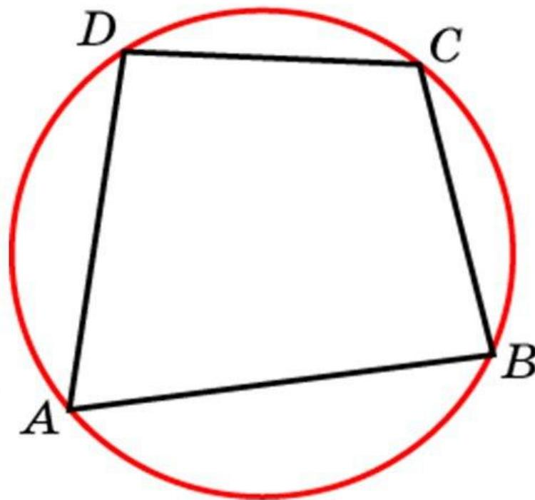
$$\angle A + \angle C = \angle B + \angle D = 180^\circ$$
