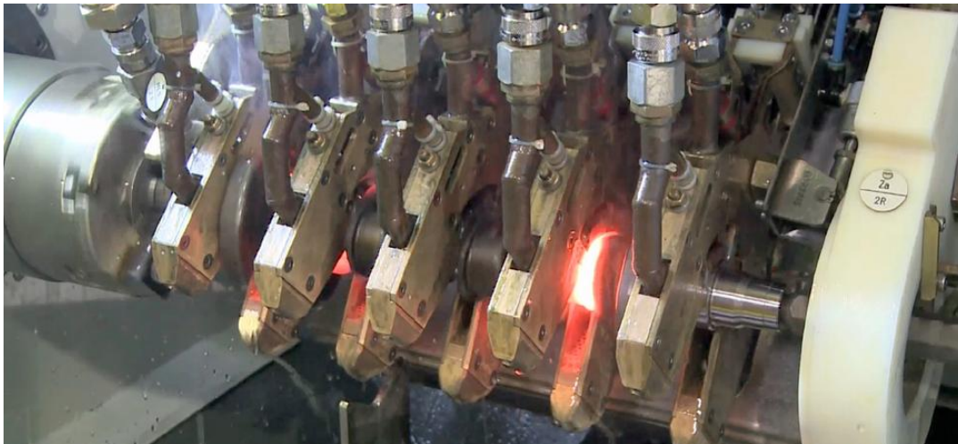
Hardening with high-frequency currents
