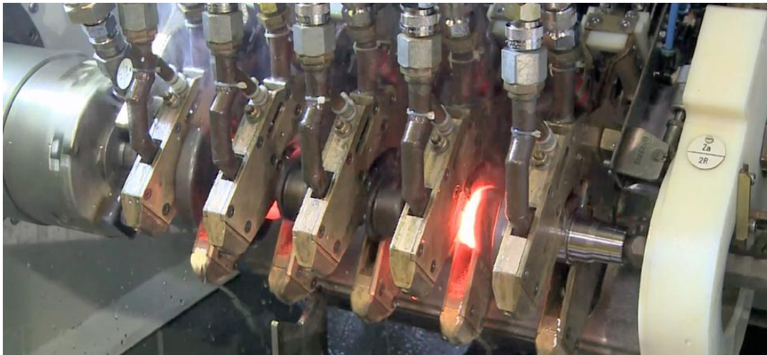
Hardening with high-frequency currents
