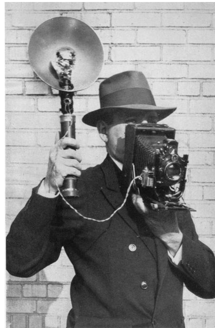
Ready for a speed flash. Illustration shows the speed gun using a flash bulb and hooked up to the camera.
