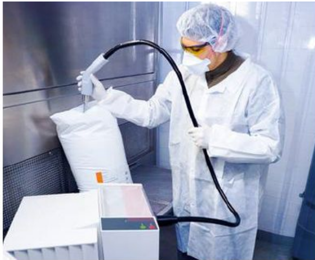
Solid fiber-optics probe
