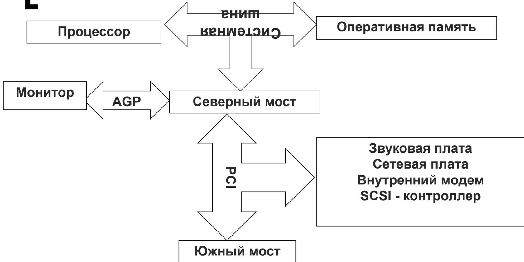
Шина PCI (Peripheral Component Interconnect bus) –
