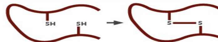
DISULFIDE BONDS IN A PEPTIDE Disulfide bonds form between thiol (-SH) groups on peptide chains
