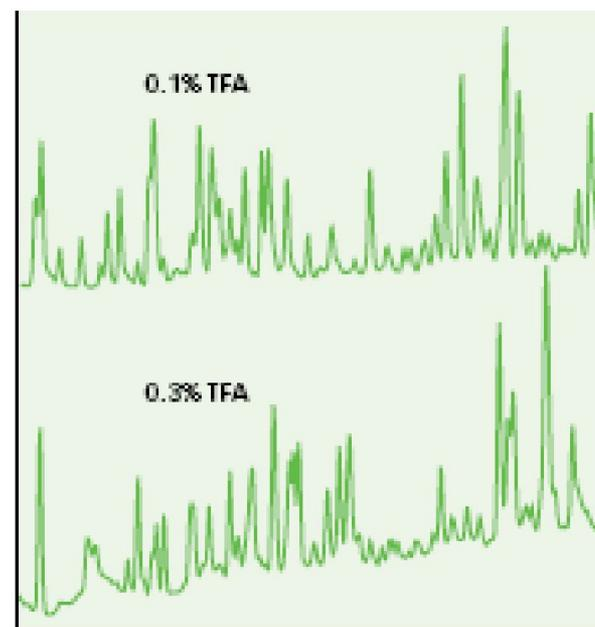
Figure 19. Significant differences in the peptide separation pattern due to differences in TFA concentration are evident. Column:  $C_{18}$  (YDAC<sup>®</sup> 218TP54). Flow rate: 1 mL/min. Eluent: Gradient from 0–50% ACN in aqueous TFA, concentration as indicated. Sample: Tryptic digest of apotransferrin. Note: Only part of the chromatogram is shown.
