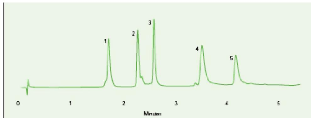
Figure 24. Column:  $C_{18}$ ,  $3\ \mu\text{m}$   $4.6 \times 50\ \text{mm}$  (YDAC<sup>®</sup> 238TP3405). Flow rate: 4.0 ml/min. Eluent: Gradient from 20–45% ACN in aqueous 0.1% TFA in 4 min. Sample: protein standards. (1) ribonuclease, (2) insulin, (3) cytochrome c, (4) BSA and (5) myoglobin.
