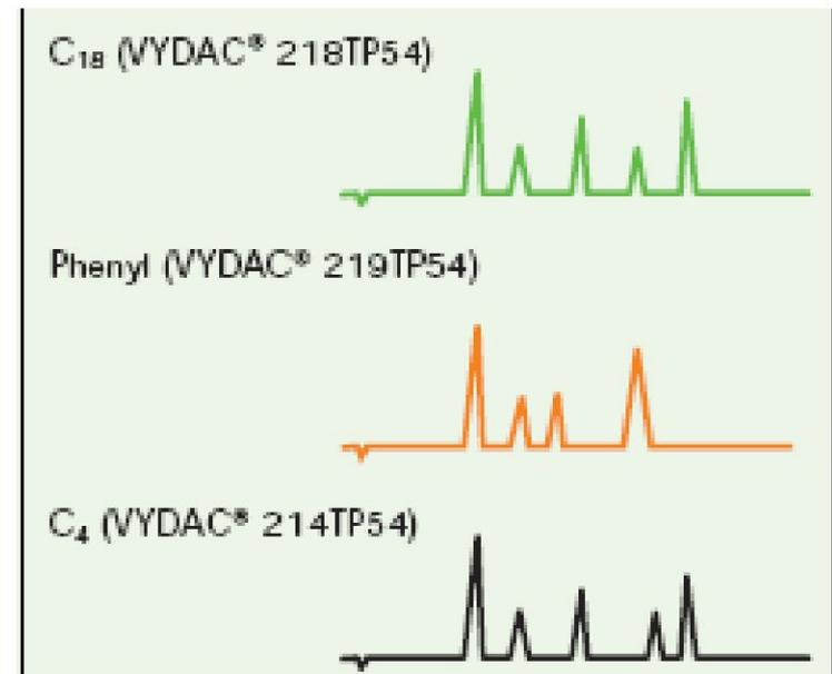
**Figure 8.** Peptide separation on different reversed-phase columns. Columns: VYDAC® 218TP54 (C<sub>18</sub>); 214TP54 (C<sub>4</sub>); 219TP54 (phenyl); Eluent: 15–30 % ACN in 0.1% aqueous TFA over 30 minutes at 1.0 mL/min. Sample: 1. oxytocin, 2. bradykinin, 3. angiotensin II, 4. neurotensin, 5. angiotensin I.
