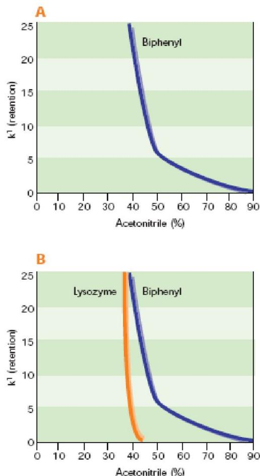
**Figure 4. A:** The retention of small molecules such as biphenyl decreases gradually as the organic modifier concentration increases because they are retained by partitioning. **B:** The retention of polypeptides such as lysozyme changes suddenly and drastically as the organic modifier reaches the critical concentration needed to desorb the polypeptide, evidence of the adsorption/desorption model of polypeptide-reversed-phase surface interactions.
