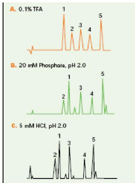
Figure 20. Elution of five peptides using TFA (A), Phosphate (B) or HCl (C) as the buffer/ion-pairing agent. Column: YDAC<sup>®</sup> 218TP54 ( $C_{18}$ , 5  $\mu$ m, 4.6 x 250 mm). Eluent: 15–30% ACN in 30 min at 1.0 mL/min; plus A. 0.1% TFA B. 20 mM phosphate, pH 2.0 C. 5 mM HCl, pH 2.0 Peptides: 1. oxytocin 2. bradykinin 3. angiotensin II 4. neurotensin 5. angiotensin I.
