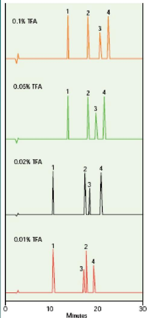
Figure 25. Column:  $C_{18}$ , 5  $\mu$ m, 4.6 x 250 mm (YDAC<sup>®</sup> 218MS54). Flow rate: 1.5 mL/min. Eluent: Gradient from 5–19% ACN in aqueous 0.1% TFA. Sample: 1. neurotensin (1–8 frag) 2. oxytocin 3. angiotensin II 4. neurotensin.
