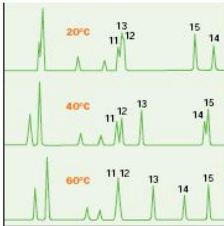
Figure 23. Column:  $C_{18}$ , 4.6 x 150 mm. Flow rate: 1 mL/min. Eluent: Gradient from 0–60% ACN in aqueous .1% TFA in 60 min. Temperature: As indicated. Sample: Tryptic digest of human growth hormone. Data from Reference 39.
