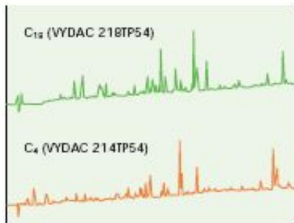
Figure 10. Columns: VYDAC® 218TP54 (C<sub>18</sub>); 214TP54 (C<sub>4</sub>); Eluent: 0–30 % ACN in 0.1% aqueous TFA over 60 minutes at 1.0 mL/min. Sample: tryptic digest of  $\beta$ -lactoglobulin A.
