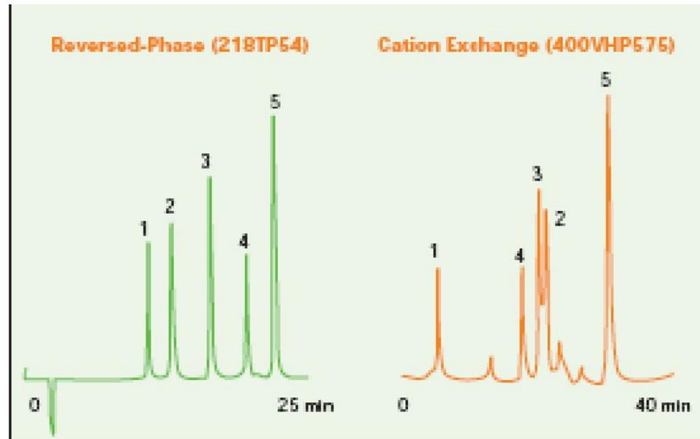
Figure D-1. *Reversed-Phase Column: VYDAC® 218TP54, C<sub>18</sub>, 5 µm, 4.6 x 250 mm Eluent: 15–30% ACN in 0.1% TFA over 30 minutes at 1.0 mL/min Strong Cation Exchange Column: VYDAC® 400VHP575, Cation exchange, 5 µm, 7.5 x 50 mm Eluent: 10 mM phosphate, pH 2.7/25% ACN; gradient from 0–0.1 M NaCl in 20 min at 1.0 mL/min Sample: 1. oxytocin 2. bradykinin 3. angiotensin II 4. neurotensin 5. angiotensin I.*
