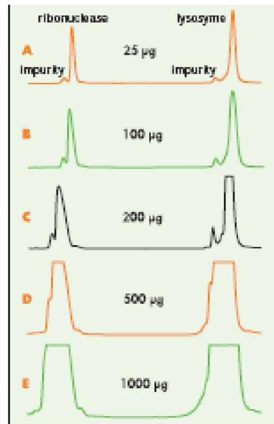
Figure 44. A. 25 µg each protein B. 100 µg each protein C. 200 µg each protein D. 500 µg each protein E. 1000 µg each protein Column: VYDAC® 214TP54 (C<sub>4</sub>, 5 µm, 4.6 x 250 mm) Eluent: 25–50% ACN in 0.1% TFA over 25 minutes at 1.5 mL/min. Sample: ribonuclease and lysozyme.
