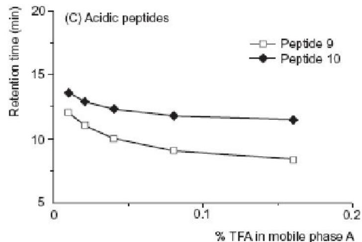
**Fig. 31.** Variation of retention time with concentration of the anionic ion pairing agent (TFA) for (A) neutral, (B) basic and (C) acidic peptides. (Work by Amersham Pharmacia Biotech Inc., Piscataway, NJ, USA.)
