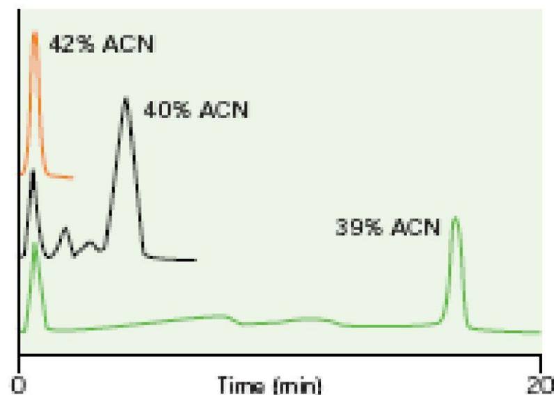
**Figure 5.** At 39% ACN, the retention time of lysozyme is nearly 18 minutes. Increasing the ACN concentration to 40% reduces the retention time by more than half, to 7.6 minutes. Increasing the ACN concentration to 42% reduces the retention time of lysozyme again by more than half, to 3.1 minutes. **Column:** VYDAC® 214TP54 **Eluent:** ACN at 39, 40 and 42% in 0.1% aqueous TFA.
