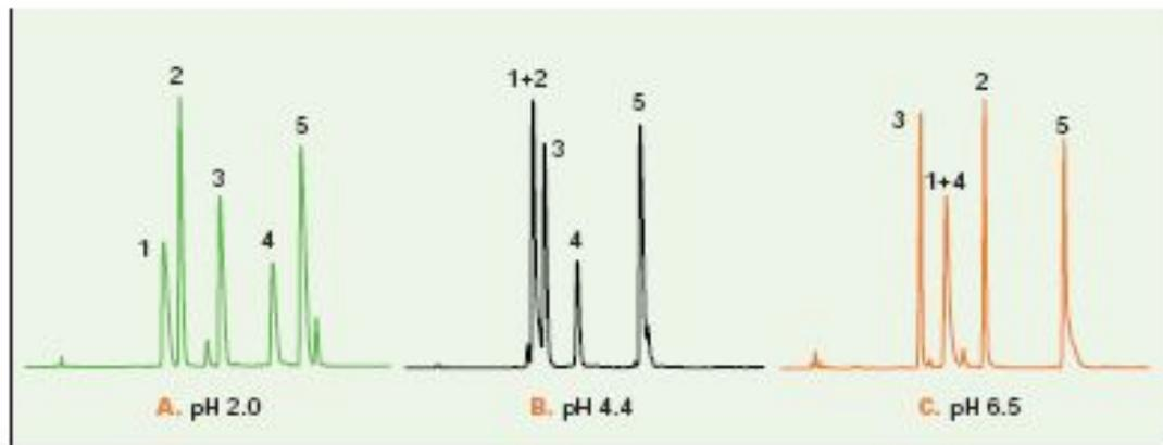
**Figure 21.** Elution of five peptides at pH 2.0, 4.4 and 6.5 with phosphate as the buffer. Column: VYDAC® 218TP54 (C<sub>18</sub>, 5 μm, 4.6 x 250 mm). Eluent: 15–30% ACN in 30 min at 1.0 mL/min; plus A. 20 mM phosphate, pH 2.0 B. 20 mM phosphate, pH 4.4 C. 20 mM phosphate, pH 6.5 Peptides: 1. bradykinin 2. oxytocin 3. angiotensin II 4. neurotensin 5. angiotensin I.
