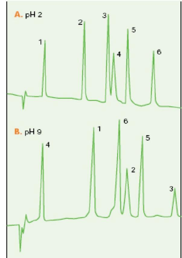
**Figure 22.** Column: VYDAC® 259VHP5415 (PS-DVB, 5 μm, 4.6 x 150 mm) Eluent: 15–30% ACN over 15 min. with A. 0.1% TFA, pH 2. B. 15 mM NaOH, pH 9. Flowrate: 1.0 mL/min. Peptides: 1. oxytocin. 2. bradykinin. 3. neurotensin. 4. neurotensin 1-8. 5. angiotensin III. 6. val-4 angiotensin III.
