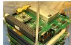
C&DH + Watchdog Board + Lithium UHF (AstroDev)
