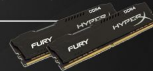
KINGSTON DDR4 DIMM 16GB KIT 2X8GB HX432C18FB2K2/16 PC4-25600, 3200MHZ, CL18, HYPERXFURY BLACK
