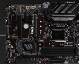
MSI Z390-A PRO RTL {SOCKET 1151, IZ390, 4*DDR4, 2*PCI-E, SATA 6GB/S + RAID, 1*M.2, ALC892 8CH, GLAN, USB3.1, D-SUB + DVI-D + DP, ATX}
