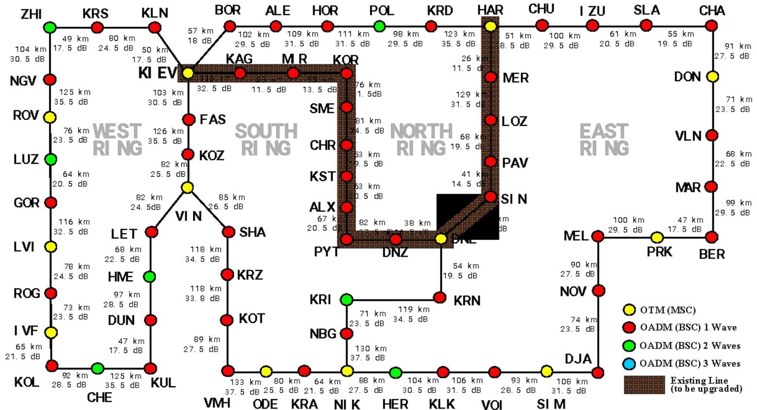
At tenuati on  $\leq$  Di stance \* 0,24dB/ km + 4dB+1.5dB
