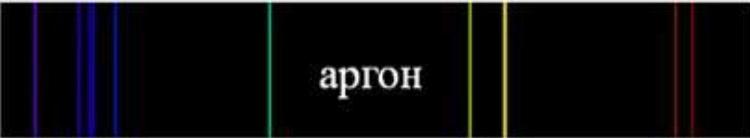
The spectrum of Argon shows a series of vertical lines on a black background. From left to right, the lines are: a double blue line, a double blue line, a single cyan line, a single yellow-green line, a single yellow line, and a single red line.
