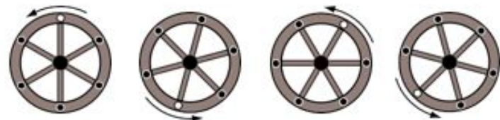
11Hz (165° per rotation): can still see direction of motion
