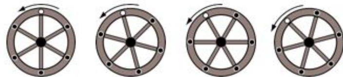
25 Hz (375° per rotation): motion forward again, but very slowly (more than one full rotation between frames)
