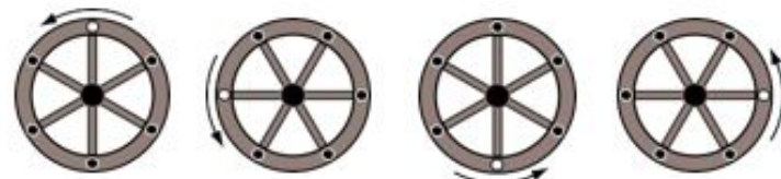
6Hz (90° per rotation): motion is clear
