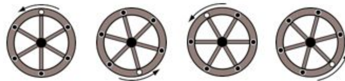
13Hz (195° per rotation): motion appears backwards
