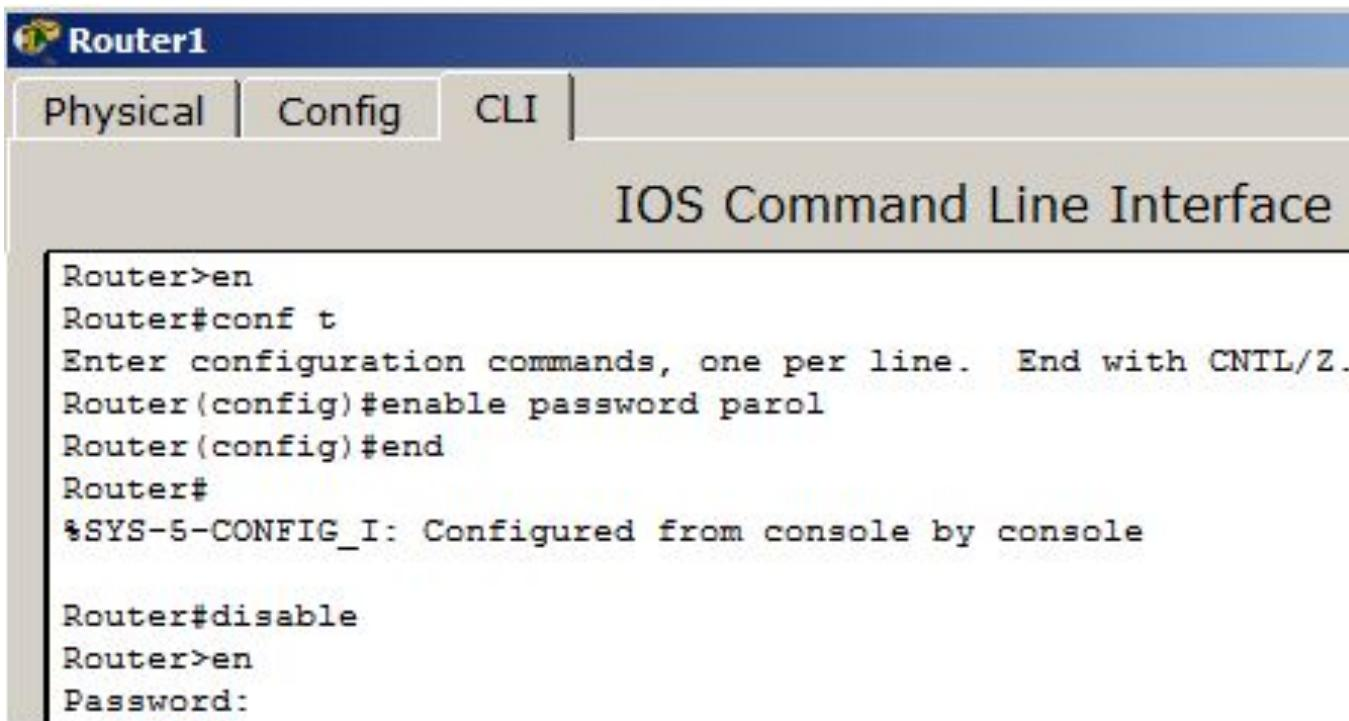
The image shows a software interface for configuring a router named "Router1". The top navigation bar has three tabs: "Physical", "Config", and "CLI". The "CLI" tab is currently selected, indicated by a red border. Below the tabs, the title "IOS Command Line Interface" is displayed. The main area contains the following command-line session:
